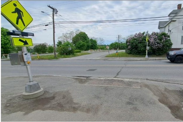
Figure 23 – RRFB and bump outs at crossing at Hardy Street and South Main Street.
