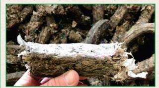
Certain components of your trash are not recyclable – but they still can be used beneficially. These materials, like plastic films and wrap, are carefully selected out of the waste stream, processed, and compacted into a briquette. Local businesses use these briquettes for internal energy generation, saving them money and helping them go green at the same time.
